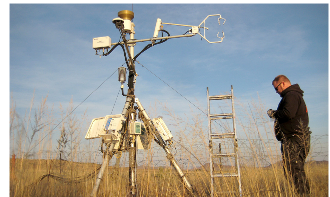
Technician maintaining the Thünen GHG measurement tower in the Karoo/South Africa
